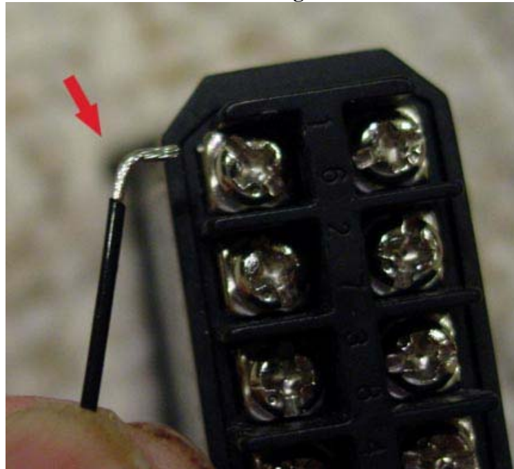
Figure 17. Bend the wire for easier insertion.
