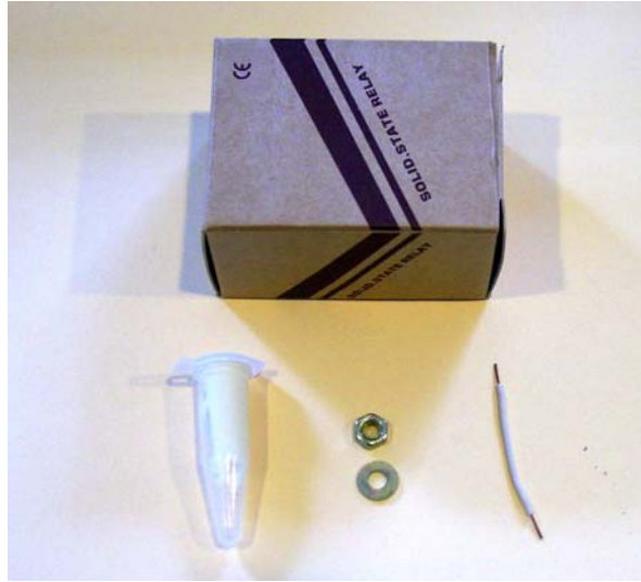
Figure 2. Solid State Relay (SSR), mounting screw nut and washer for SSR, silicone heat transfer compound (white paste in the vial) for SSR and sensor, and RTD jumper cable (see section D part 3).
