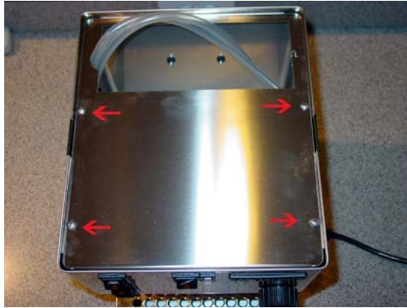
Figure 9. Top panel. Red arrows indicate the screws that hold the top panel.
