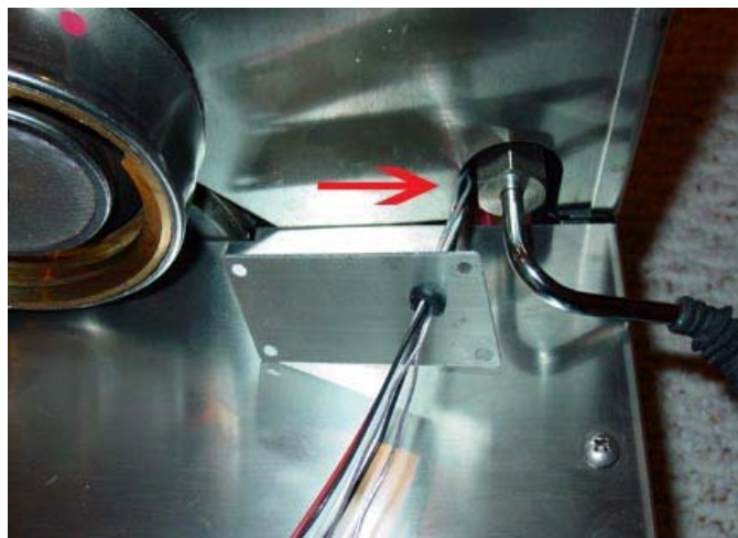
Figure 15. Cables going through the back panel of the controller box.
