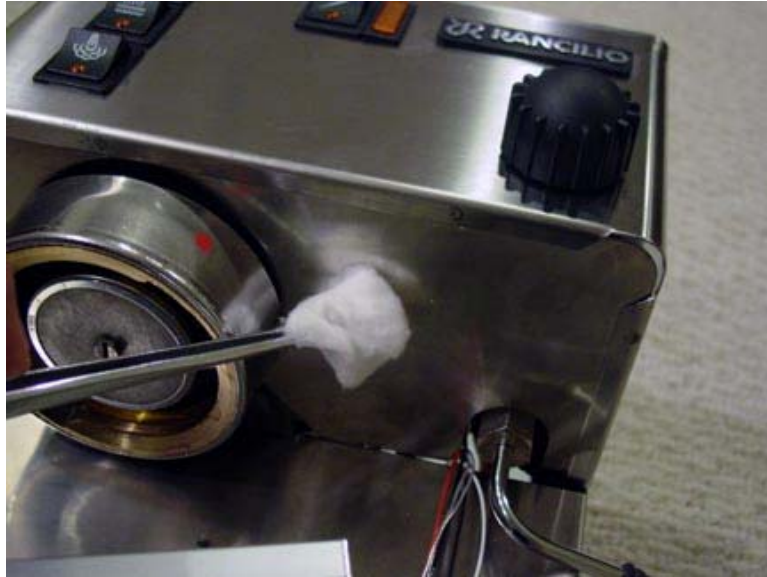
Figure 20. Cleaning the box mounting area with alcohol.
