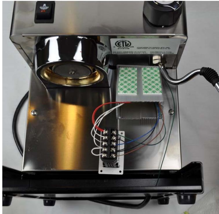
Figure 26. Connecting the wire to controller
