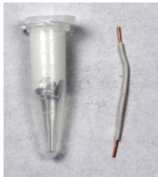
Figure 11. Left, silicone heat transfer compound (white paste in the vial) for SSR and sensor, Right, RTD jumper cable, white.
