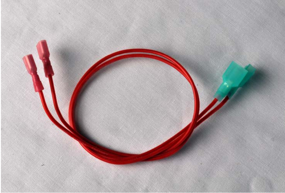
Figure 3. Pair of red cables for connecting SSR output to the cables that used to be on the brew thermostat. They are terminated with female disconnect on end and male disconnect on the other.
