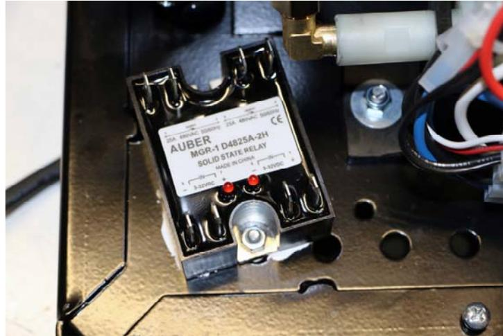
Figure 4. Mount the SSR to the location where the timer was originally installed.
