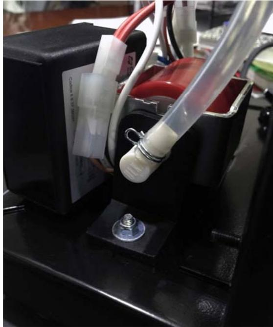
Figure 2. Mount the timer to the right side (also see Figure 5). Please note location of the white connector on the red cable.
